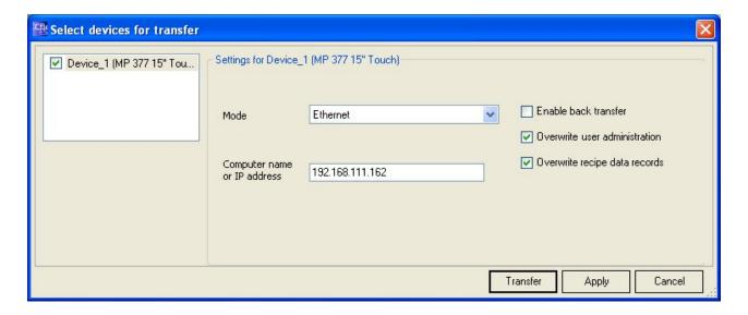
Ensure that you have clicked the "Transfer" button in the Loader menu on the Siemens panel. Then, simply click the Transfer button here to begin the transfer process. Depending on the size of your WinCC Flexible project, this transfer could take several minutes.
