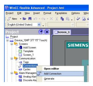
This will open the Connections editor and will add a new connection to the list that will default to using the "SIMATIC S7 300/400" Communication driver. Clicking on that field will open a list of drivers to choose from, and we want to choose the OPC driver, as shown below.
