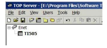
An Array tag for the Simatic 505 Ethernet driver in this example would look like: Enet.TI505.V10[10]@Word
