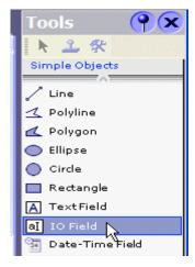
You can now return to the screen in the main panel and click and drag to create an IO field as large as you would like, as shown below.
