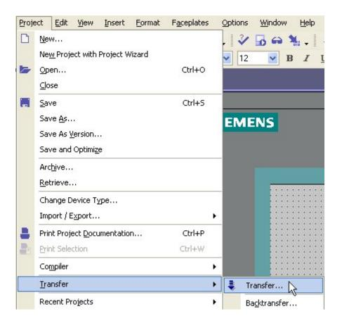
This opens the Transfer Settings dialog box, where you will select your mode of connection to the Panel and input the correct communications settings.
