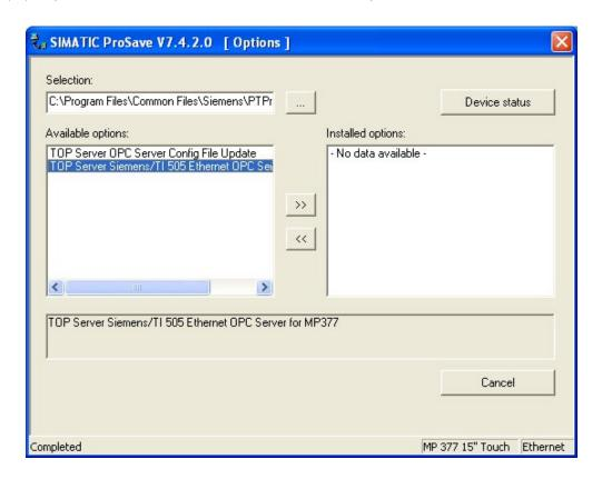
When the correct path is selected, available options will be listed, which will depend on which TOP Server drivers for Siemens panels you have installed. For this example, only a single driver was installed, so there will be two options available: the actual TOP Server Driver/Server and the Config File Update.
