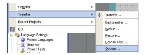
This will open the ProSave dialog box, which allows you to browse your computer for files to transfer to your Siemens panel (separate from your WinCC Flexible HMI project).
