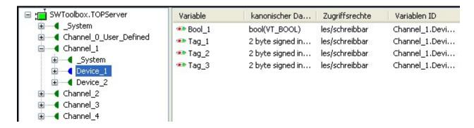
To select a tag, simply highlight it and click the Check button at the bottom of the browser. This fills the Symbol and Address fields with the proper fully qualified OPC item name, as well as changing the Data type to match that of the tag in TOP Server, as shown below.
