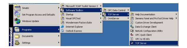
It is important you run the OPC Server installer version for Siemens Panels after you have installed the TOP Server Desktop version, since that installer installs the driver CE runtime binaries and advises WinCC Flexible of the presence of the drivers. This paper will use the terms OPC Server and TOP Server interchangeably though out this document. Also, if you are using the UCON driver, it is important that you install the TOP Server and not the UCON Standalone Server.
