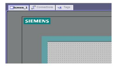
If a screen is not open, you can open the screen by double clicking on it in the Project menu under "Screens" as shown below.
