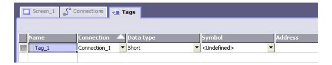
The Name field can be given any representative name you would like. This will be the name of the tag you will see as you configure your HMI Screens later. If the default connection does not match the OPC connection you created, you can change the connection by clicking the dropdown under that field, as shown below.
