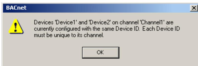
If an invalid Device ID is written to the "\_DeviceId" device System Tag, this message will not be received. Such configuration changes will cause communications with that device to fail.
