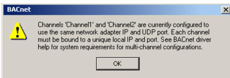
This message will not be displayed if an invalid adapter selection is written to the "\_NetworkAdapter" channel System Tag; however, such configuration changes will cause communications with all devices on that channel to fail.
