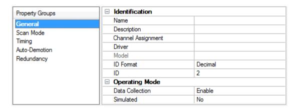
**Data Collection**: This property controls the device's active state. Although device communications are enabled by default, this property can be used to disable a physical device. Communications are not attempted when a device is disabled. From a client standpoint, the data is marked as invalid and write operations are not accepted. This property can be changed at any time through this property or the device system tags.
