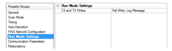
**CS and TS Writes**: Select how the device performs writes in Run mode. The default setting is Fail Write, Log Message.
