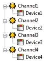
Each device has now been defined under its own channel. In this new configuration, a single path of execution is dedicated to the task of gathering data from each device. If the application has 512 or fewer devices, it can be optimized exactly how it is shown here.
