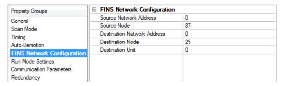
**Source Network Address**: Specifies the address number of the source network (the computer running the driver). The Source Network Address is sometimes referred to as SNA in Omron FINS documentation. The valid range is 0 to 127. The default setting is 0.
