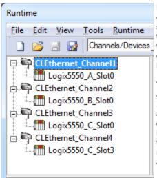
Each device has now been defined under its own channel. In this new configuration, a single path of execution is dedicated to the task of gathering data from each device. If the application has 256 or fewer devices, it can be optimized exactly how it is shown here.
