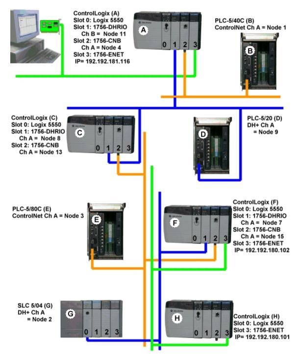
**Example 1** Logix5550 to PLC-5 via DH+ Gateway.
