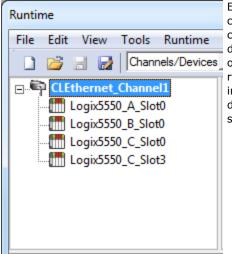
Each device appears under a single channel, called "CLEthernet\_Channel1". In this configuration, the driver must move from one device to the next as quickly as possible in order to gather information at an effective rate. As more devices are added or more information is requested from a single device, the overall update rate begins to suffer.
