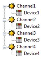
Each device has now been defined under its own channel. In this new configuration, the OPC Server can dedicate a single path of execution to the task of gathering data from a single device because each has its own dedicated channel. If the application has 8 or less devices it can be optimized as displayed.
