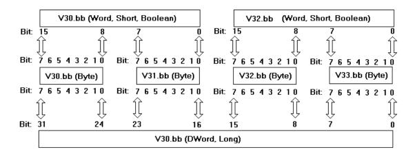
**Note**: V30.10@bool, V30.2@byte, and V30.26@DWord all reference the same bit in the controller.
